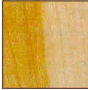
A closeup shows typical grain patterns found in plain sliced natural birch veneers.
