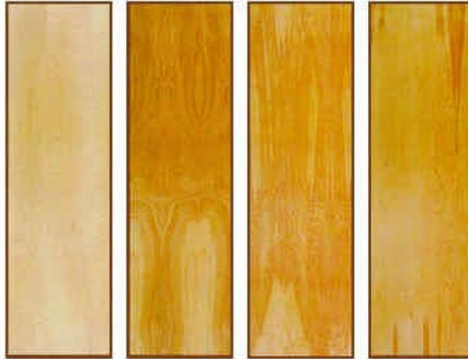
The examples shown here are of typical grain and color variations found within “A” grade (book matched) rotary cut natural birch veneer. Again, they do not represent the widest range possible. Rotary natural birch is also available in “B” grade (pleasing matched) with the face made up of veneer leaves from different logs.
