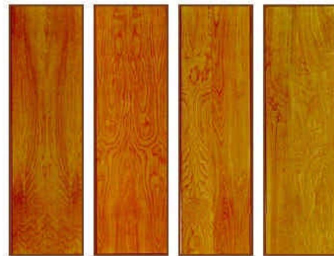
***The two examples at left are "A" grade rotary cut red birch (book matched) and the two at right are "B" grade rotary cut red birch (pleasing matched). As in other examples, they do not represent the entire range of color and grain variations that can be expected.***
