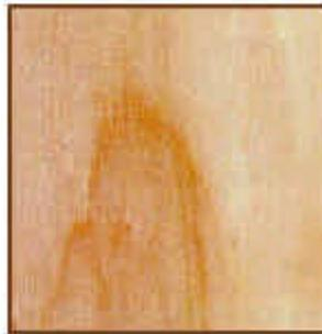
A close-up reveals the grain pattern in a rotary cut natural birch veneer.
