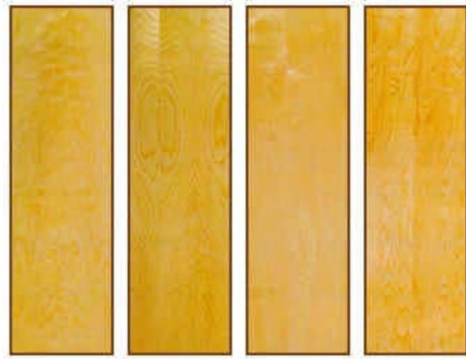
***Rotary cut white birch veneers, like their red counterparts, can come in "A" grade (the two at left) or "B" grade (like the two examples at right).***
